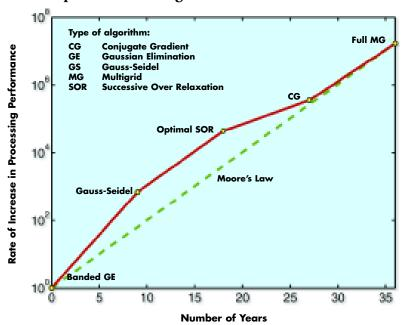
The relative gains in some algorithms for the solution of an electrostatic potential equation on a uniform cubic grid compared to improvements in the hardware (Moore's Law).
